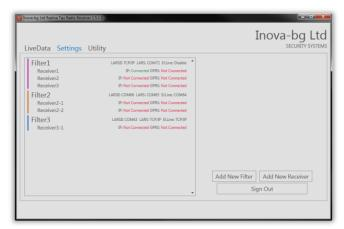
Depending on your system you can add as many filters and receivers as needed. Each filter acts like new/separate radio system with its own receivers as receiving points.
