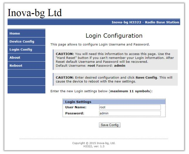
In Login Config menu you can change the username and password used to access the web-server. Maximum length for both fields is 11 symbols. If you forget your credentials you can perform a hardware reset to recover default settings:
