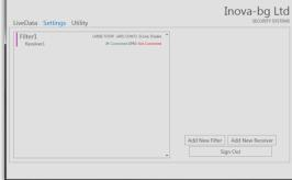
After a filter is created new Receivers can be added. Click "Add New Receiver" and change the receiver settings corresponding to your system. Note that every receiver should have a different TCP Port.
