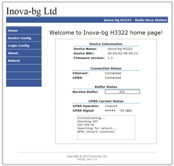
On the homepage you can find main information about the device and the current status of the connections and also the status of the GPRS network connection and the signal strength.
